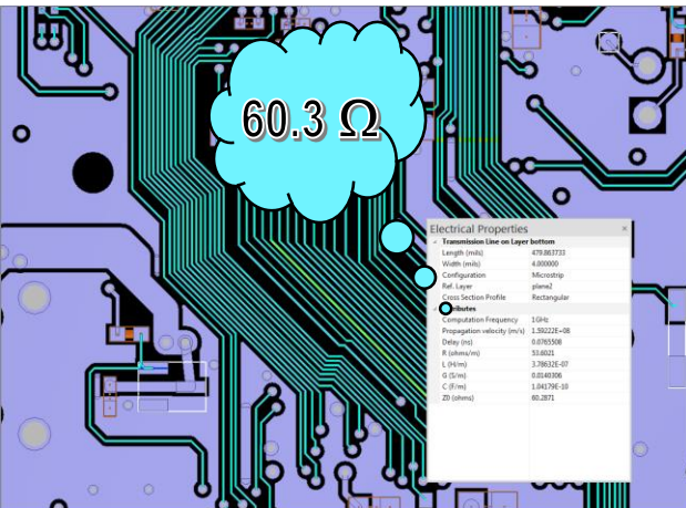
Single Ended Zo Without Trace-Trace Coupling Without Conformal Soldermask
